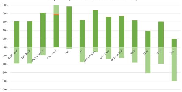
Hot-spot analysis of voestalpine cold-rolled steel strip
